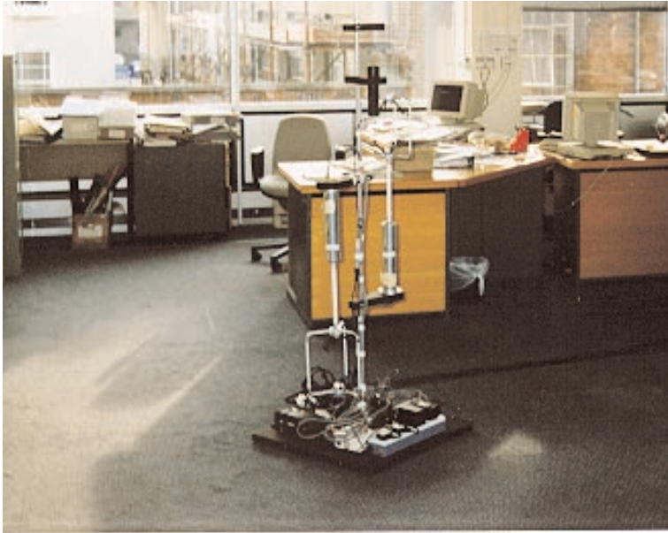
Figure 6 Monitoring equipment mounted on a mast and in place in an office
