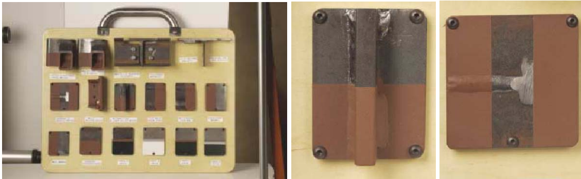
Figures 17, 18 and 19: An AESS Sample Board, Fillet Weld Sample, Groove Weld Sample 5
