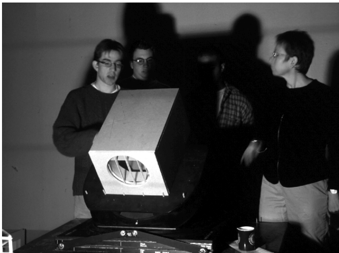
model on heliodon under summer conditions
