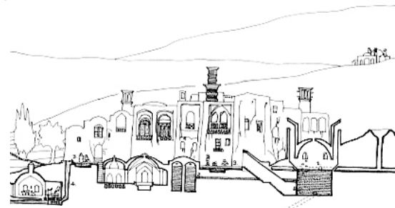
Figure 10 Section through the village of Khoranaq, Yazd, showing the passage of the water from clean to dirty uses.
