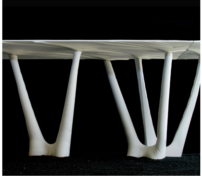
[Figure 13] Mark West, Fabric Formed Cast Models
