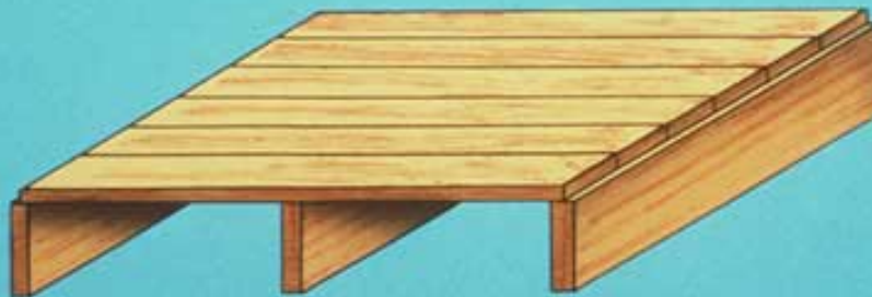
TWO SPAN CONTINUOUS PATTERN
