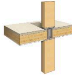
partial encapsulation during construction
