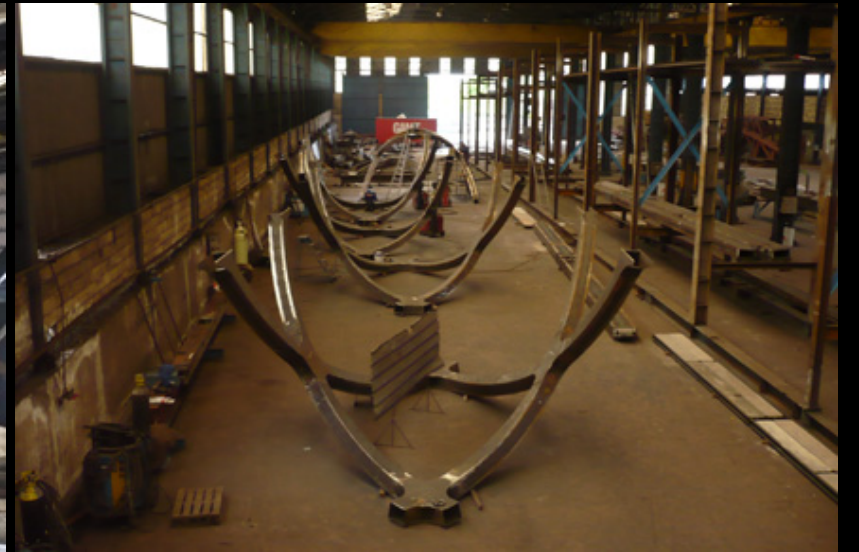
Images of the steel fabrication. All custom sections whose curvature was created via brake forming. Welds all ground smooth. AESS4
