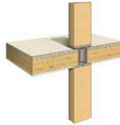
partial encapsulation during construction
