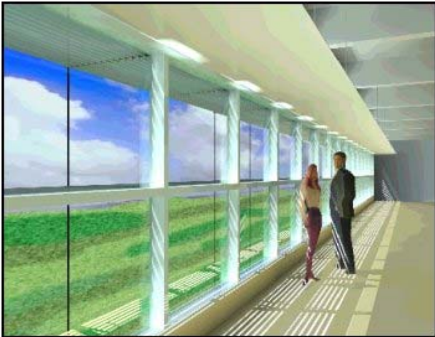
Light shelf designed for BC Gas Operations Centre in Surrey BC.
